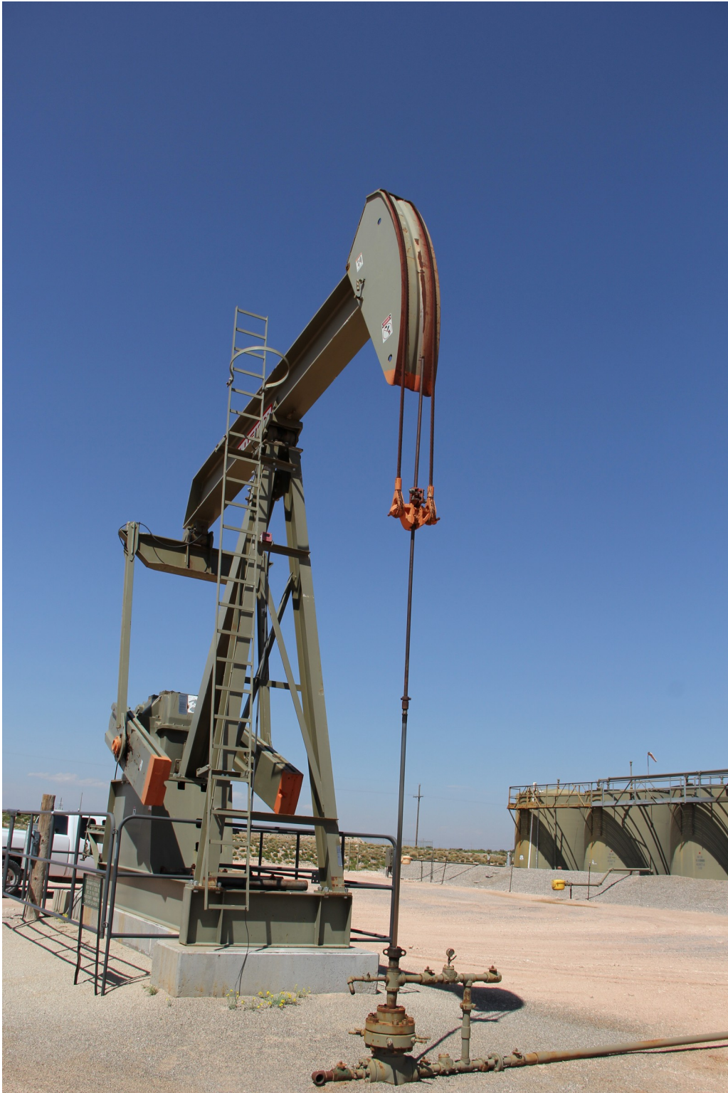
Pumpjack in an oil and gas field. (Bureau of Land Management, public domain, via Wikimedia Commons.)
