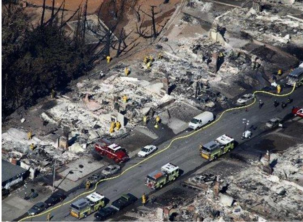
A 2010 explosion in San Bruno, CA pipeline flattened a neighborhood and killed 8 people ( http://blog.sfgate.com/energy/2013/05/15/pges-900-million-san-bruno-tax-break/ ). This explosion occurred after increased pressure in the line weakened some poorly welded seams.
